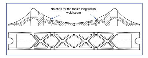
Due to its composition, this composite support can come directly into contact with the tanks and comply with standard 87/404/CE.
