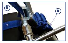
**4** - With a 19 mm wrench, tension the strap to around 60 newtons/metre, then cut (\*) the strap on each side of the CLIP at a distance of 30 mm (min.).
