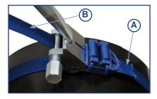
**3** - Position the tensioning tool and put the strap (longest side) into the slot of the tool.
